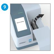
Remove and immediately discard the used test cartridge. Close the lid manually when the analyzer is not in use.
