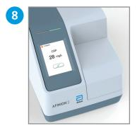
Record the result when it appears on the screen. Touch  $\checkmark$  to accept. The lid opens automatically.
