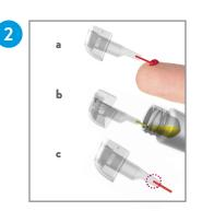
Fill the capillary completely (c) with patient sample (a) or control (b). Do not wipe off the capillary.
