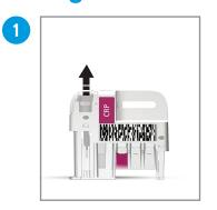
Pull the sampling device straight up from the test cartridge.
